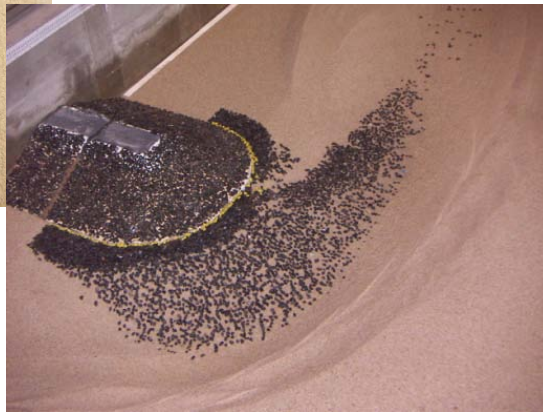
Abutment test Convectional scour protection UBI flume (Portugal)
