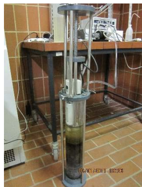
Transport to the lab to determine mass erosion at high shear stress (worst case)
