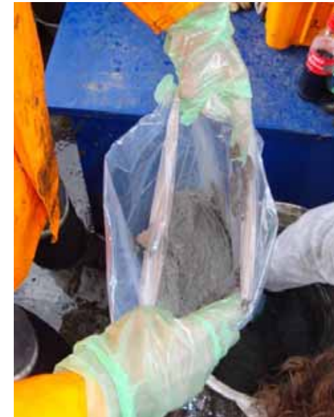
The tracer was placed in soluble bags
