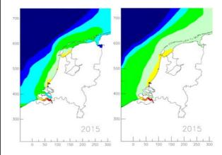
**Fig. 2:** Prognosis of TBT concentrations in 2015, without (left) and with (right) effect of sediment accumulation. Orange and red colours indicate concentrations exceeding the WFD standard.
