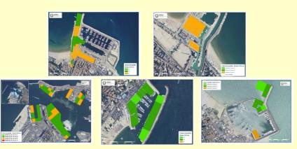
By means of a regional integrated solution these ports can use their dredged sediments for beach nourishment, open water disposal and to fill a CDF in the port of Ancona
