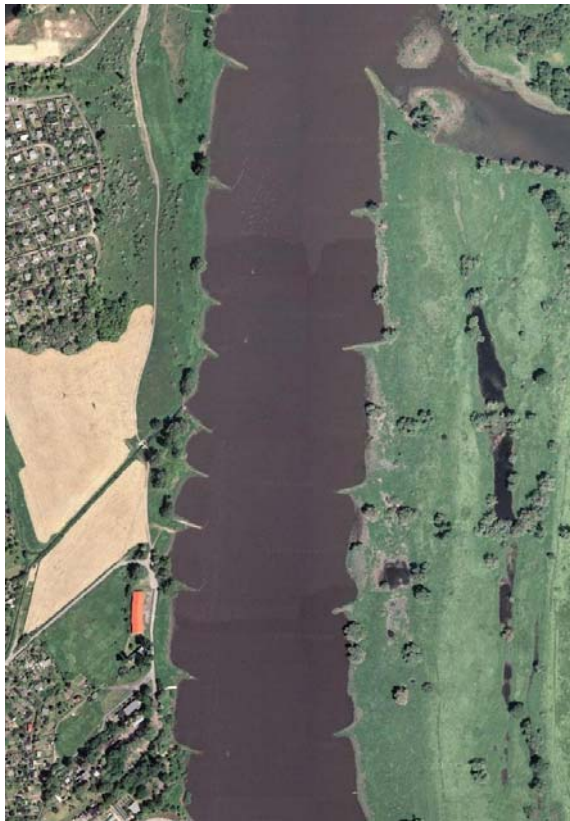
Fig. 1: Section over the River Elbe near Magdeburg, trained by groynes.
