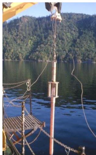
Gravity core sampler
