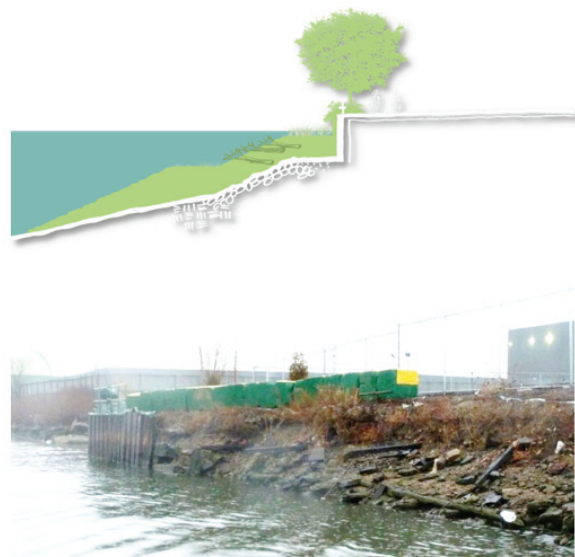
Fig. 1a: Example restoration approach adjacent to bulkhead shorelines. In the conceptual section, the original shoreline is shown in white, and enhancements are drawn in green. The photograph is included as pre-restoration context.
