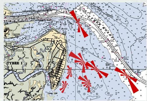
GTRAN calculates transport direction and magnitude at multiple locations over complex domain. Defines transport pathways and dominant transport directions due to currents, waves, at DC
