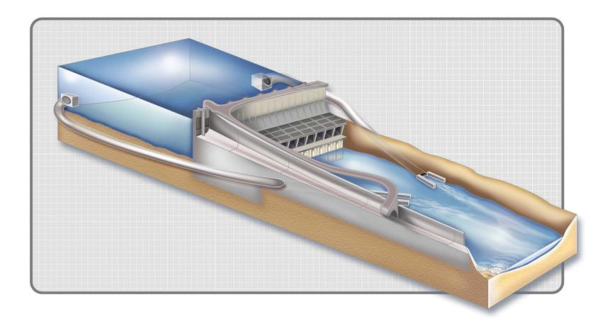
• Génissiat dam includes 3 hydraulic outlets located at 3 different elevations
