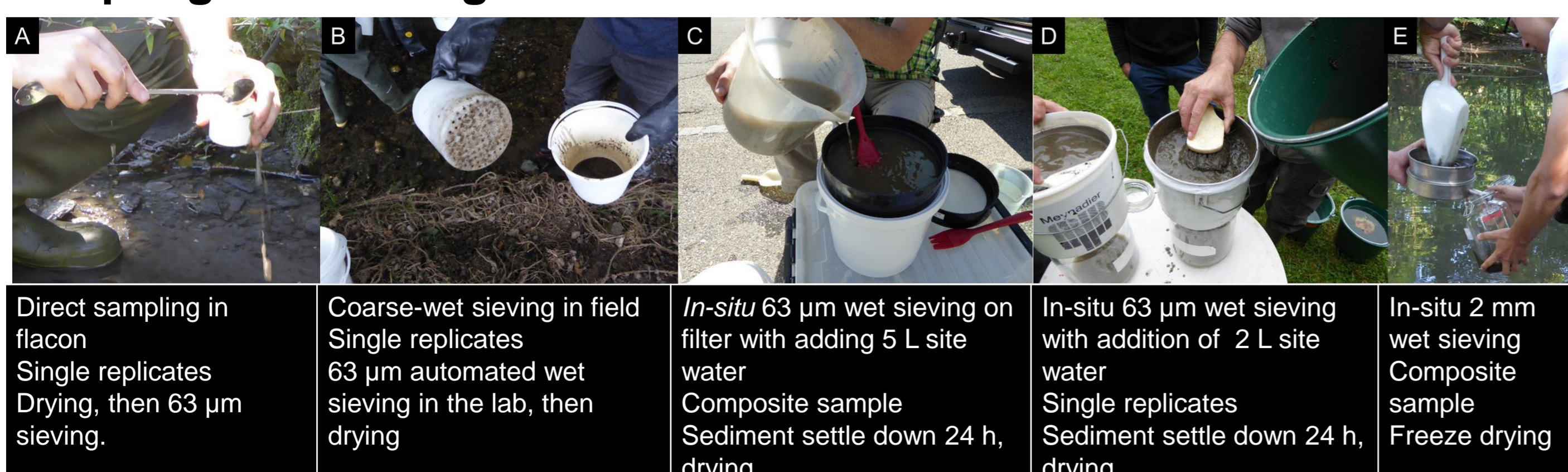
Fig. 4 Illustration of cantons with different sampling methods that include different sampling devices, sieving procedure and pretreatment.
