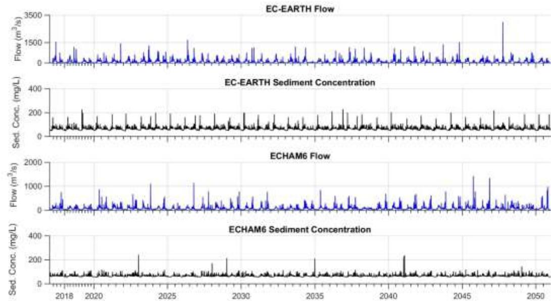
The FEST-WB-ERODE model output for extreme scenarios expressed in terms of flow and total sediment load have been used here as boundary condition for the simulation of the future sediment deposition dynamics in the Pallanza Bay, using EFDC
