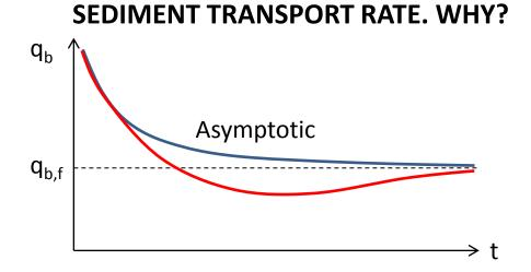
**Hypothesis:** differences in mobility of the coarse and fine grain classes for the given flow conditions.
