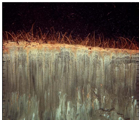
Fig. 2: SPI image from the Oslo harbour area. The sediment surface is recolonized of small tube building polychaet after a capping.
