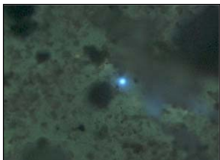
Fig. 1: A 5 µm fluorescent tracer particle at ×20 magnification in sediment.
