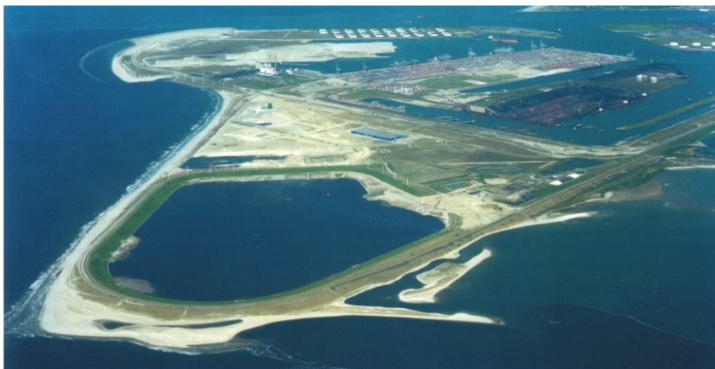
Figure 2-2: The Slufter – a confined disposal site for contaminated dredged material
