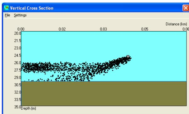
**Fig. 1:** Simulation of deposition of capping material through a hose from a moving barge. A diffuser arrangement has been mounted at the end of the hose. The model simulates the deposition of the capping material. The figure shows the particle material discharged and also sinking down on the sea floor. The diffuser is moving to the right.
