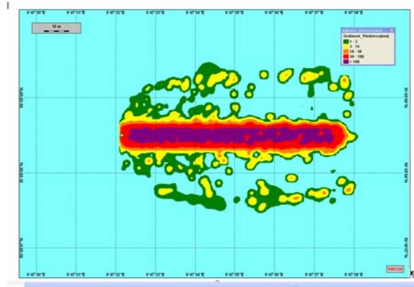
**Fig. 2:** Deposition of capping material on the sea floor. Example from a case where a diffuser is towed across the sea floor.
