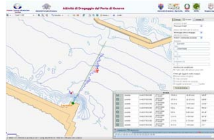
Fig. 2: Authoring tool: real-time visualization of the current flow obtained from acoustic measurements through ADCP mounted on the dam at the port of Genoa.
