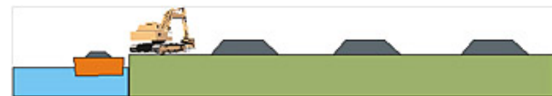
Fig. 4: Selective processing of dredged sediment loads (left) in canal-side treatment plant: uncontaminated, direct shipping to reuse site; low contamination: dehydration or landfarming until reuse (1); medium contamination: treatment and separation (2); high contamination: concentration and disposal as hazardous waste (3).
