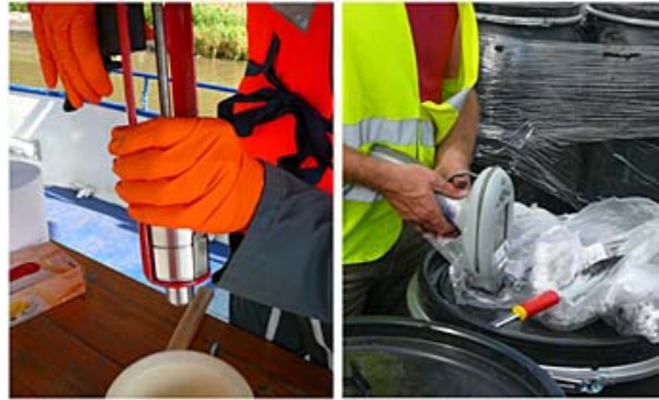
Fig. 1: On-site sample preparation (left) and pXRF analysis (right)
