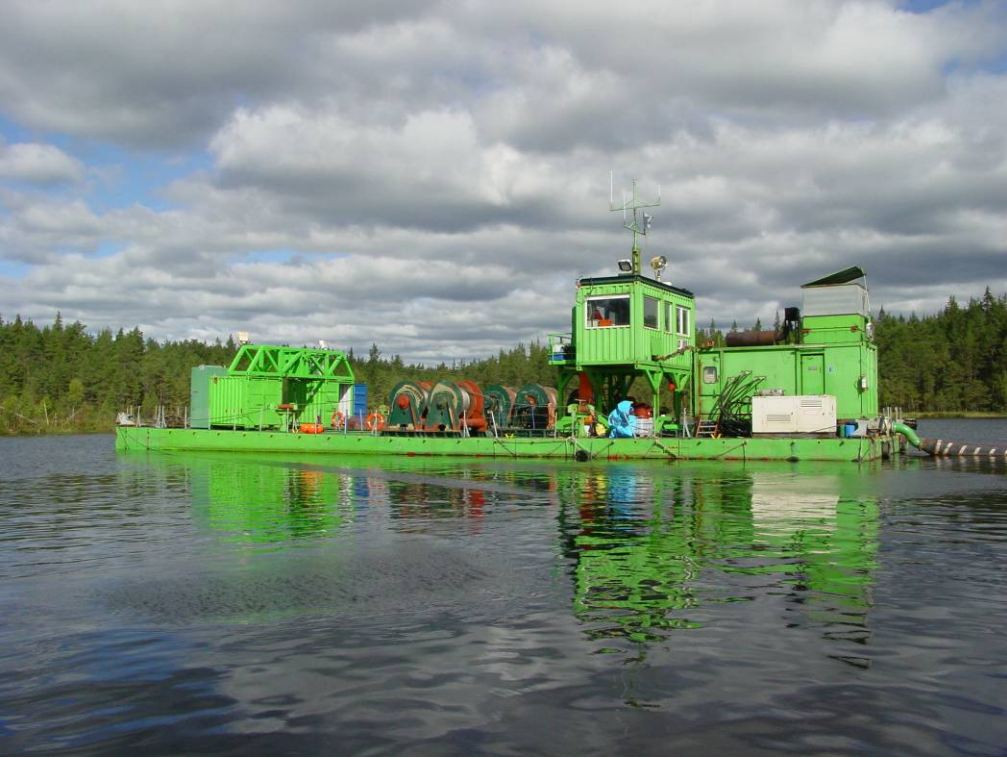
Picture of the environmental dredge at work at the Svartsjö lakes.
