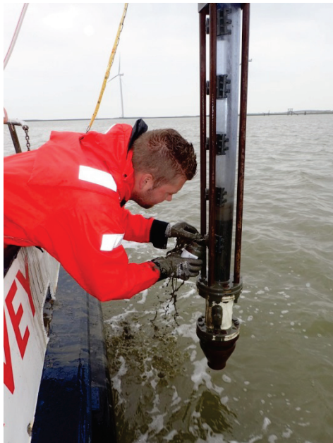
Figure 2: 'Sludge Sampler' for sampling the sediment
