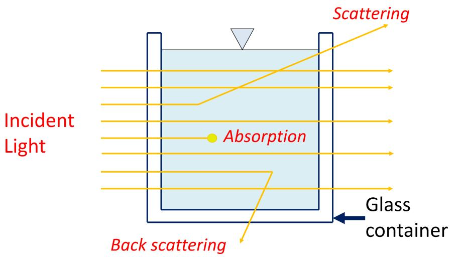
Total light (beam) attenuation = absorption + scattering: c = a + b
