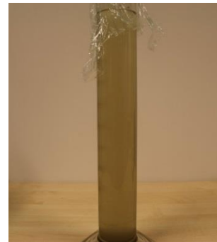
Fig. 1: Settling column, sediment, normal light.
