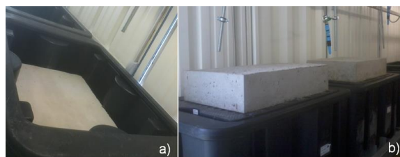
Fig. 1: Photograph of experimental set up allowing simulating a) water immersion for foundation layer blocks b) water runoff for road surface blocks
