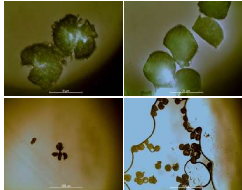
Figure: The difference between aged and non-aged MPs (63-75 \mu\text{m} ) under the microscope. The two pictures on the left are aged for 4 days while the two pictures on the right show MPs when taken out of the packaging tubes.
