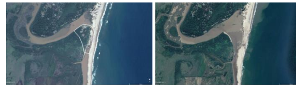
Fig. 2: The white area on the image (above left) indicates the area of dredge spoil to be removed, while the image on the right shows the sediment removal almost complete at the end of May 2017.
