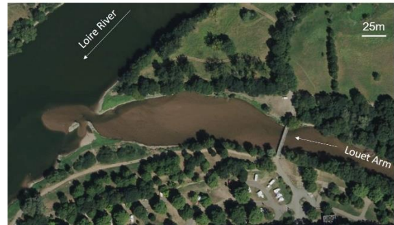
Fig. 1: Confluence between Loire River and Louet arm after downstream weirs removal (data @2018 Google)
