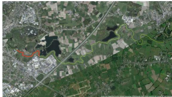
**Fig. 1:** Environmental quality of sediments: green being acceptable as building material, red meaning there is exceedance of certain parameters.
