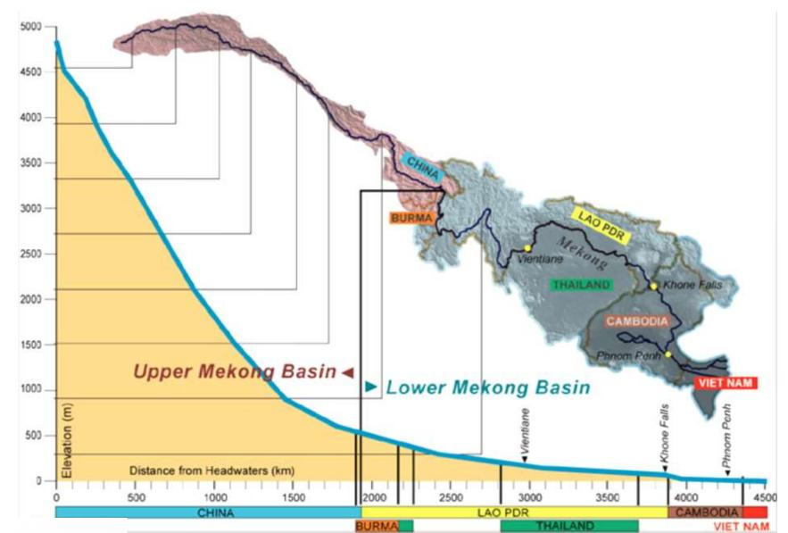
In the Chinese section of the river (upstream), 7 dams have turned the river into a series of reservoirs, cutting off sediment supply from the upper basin, which formerly supplied 50% of the river's sediment. *More dams planned upstream.*
