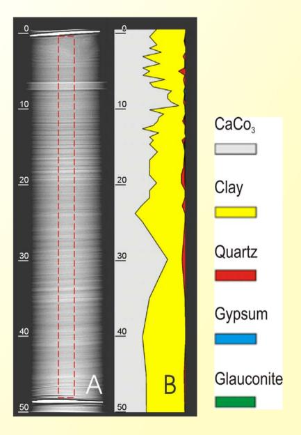
The BS 600 core consisted of unconsolidated detritic material: a mixture of clay and calcium carbonate.
