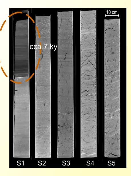
CT image of a core consisting of unconsolidated sediments collected on the Western Black Sea continental platform slope at a depth of 500 m indicating the onset of euxinic conditions
