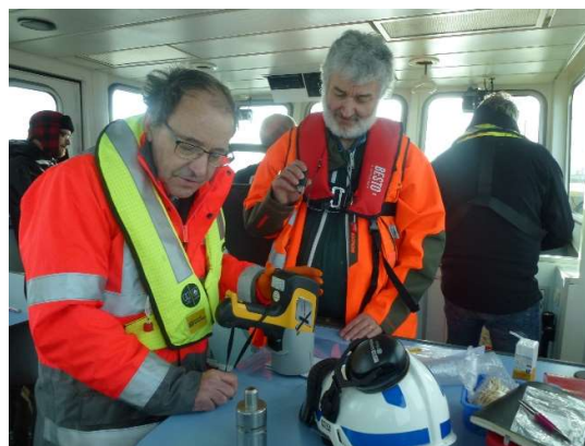
Fig. 1: On-board pXRF analysis of dredgings.
