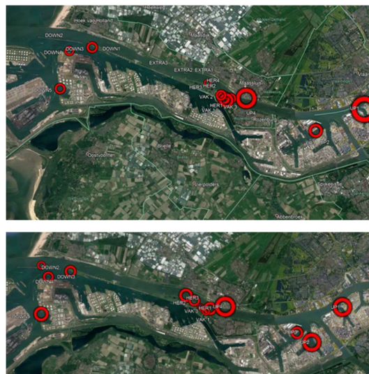
Fig. 1: Top, initial T_0 Lanthanum enrichment in the NWW (as compared to marine sediment). Bottom the NWW Lanthanum enrichment after 9 months compared to T_0 .
