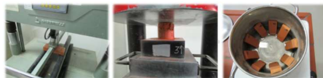
Determination of bending strength, compressive strength and water absorption
