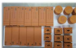
Water absorption and shrinkage upon firing temperature (results from gradient kiln) Samples fired at 950 °C
