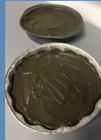
7.5% Portland cement Immediately after mixing
