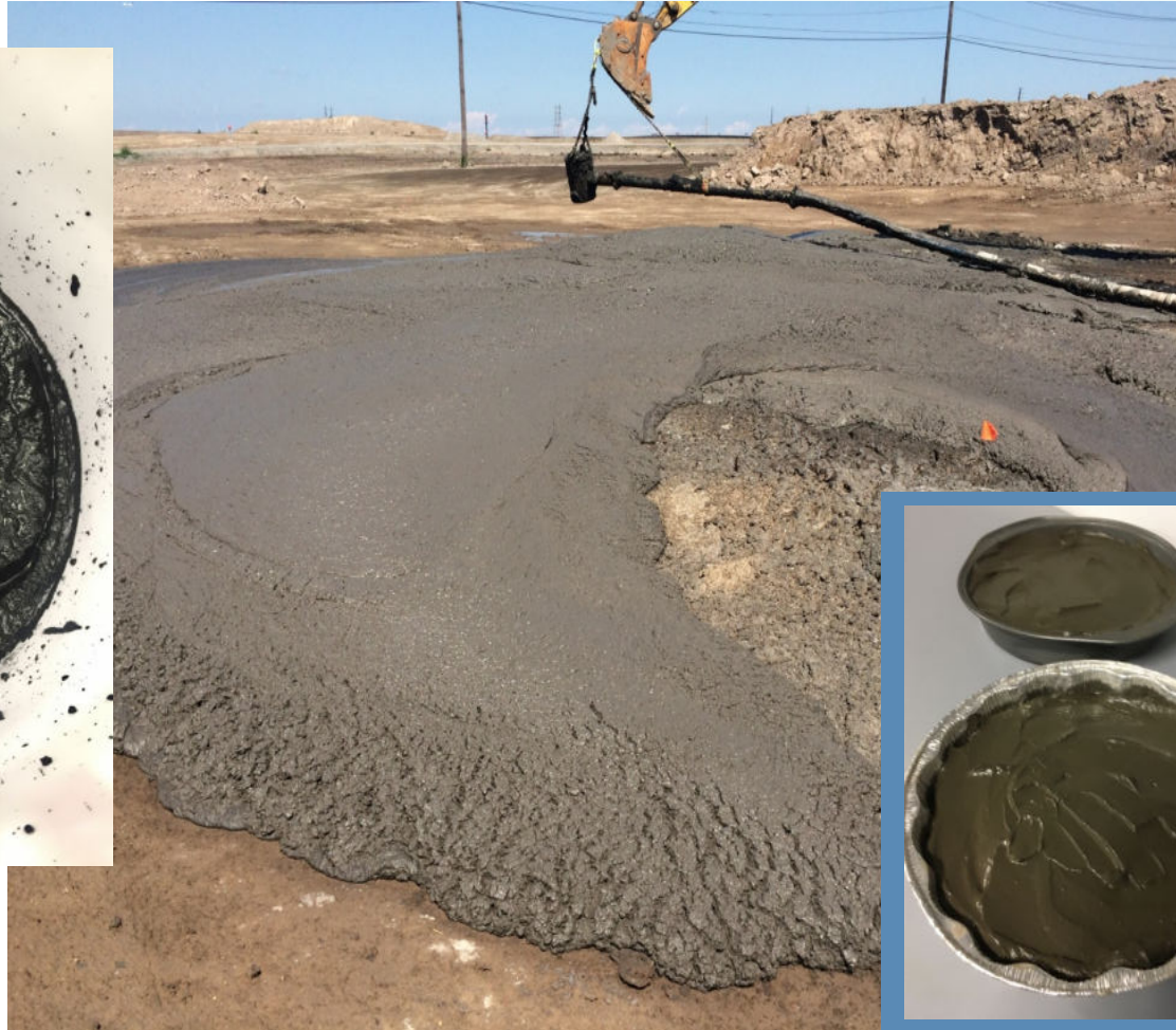
7.5% Portland cement Immediately after mixing
