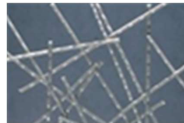
Macrofibres - mainly used as reinforcement in shotcrete
