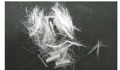
Microfibres - mainly used as fire protection in shotcrete
