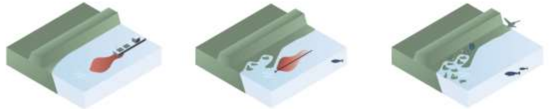
Figure 3. Sediment is reallocated in water at a strategic location, Tidal flow and waves transport the sediment to the final location (in this illustrative case, for wetland restoration in front of a sea dyke, with consequential reduction of flood risk).
