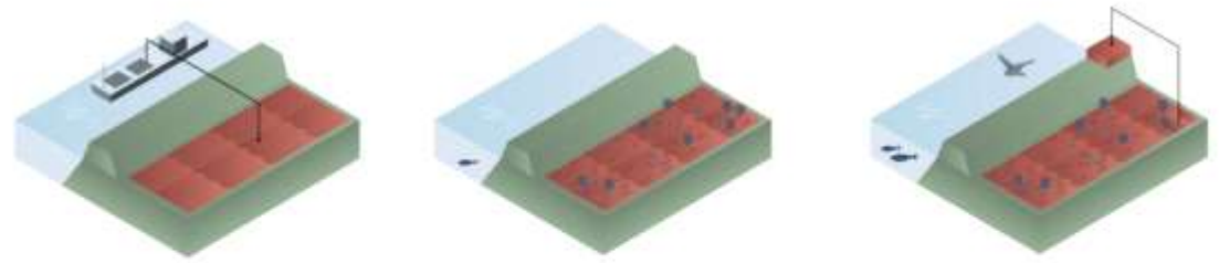
Figure 1. Sediment is deposited on land (in this illustrative case, in drying cells), possibly treated and reclaimed for other subsequent beneficial uses (in this case for dyke reinforcement).
