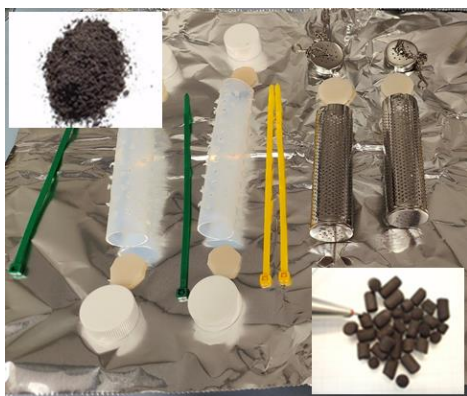
Fig. 1: Variations of in situ microcosm cages containing carrier materials for 13 C-labeled pollutants.
