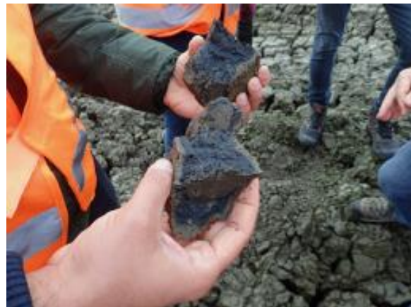
Fig. 1: Oxidation of organic matter at edges of sediment desiccation polygon, Kleiriperi, Delfzijl.
