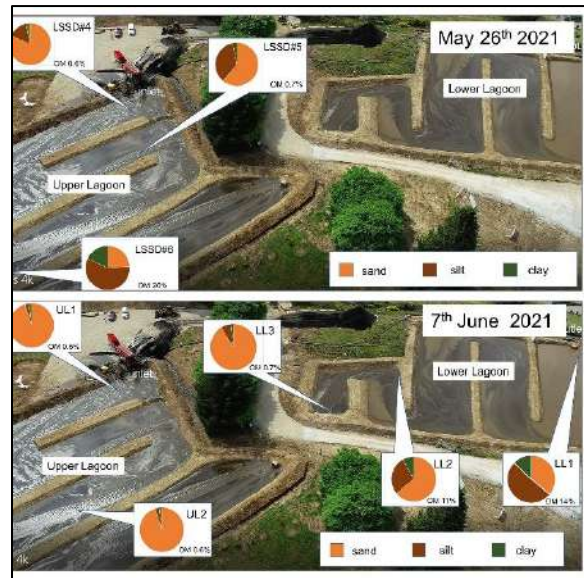
Fig. 2: Sediment segregation within lagoons.
