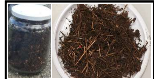
Soil as-is and mixed with straw
