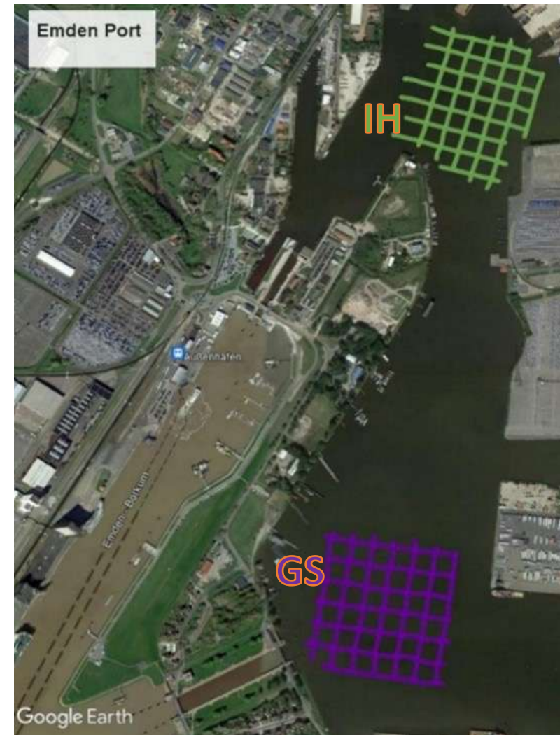
Port of Emden monitoring lines, the lines intersections are the measuring points.
