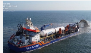
Trailing Suction Hopper Dredger
