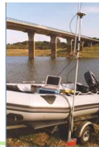
Boat Single beam echosounder RTK GPS
