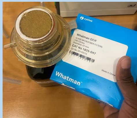
Filtration with Glass Microfiber filter
