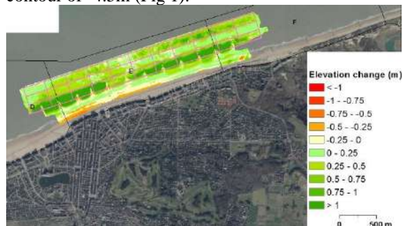
Fig. 1: DEM of difference between pre (10/2023)-post (03/2024) nearshore nourishment surveys.
