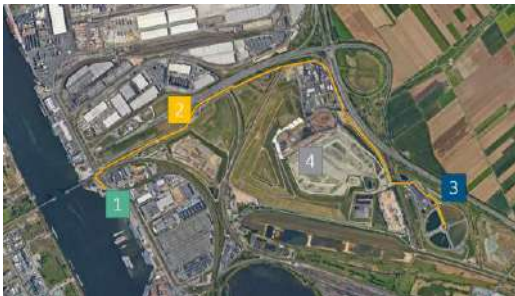
Fig. 1: AMOARS dewatering installation: 1) Underwater disposal cell and sand separation, 2) piping system, 3) dewatering and water treatment site, 4) storage.
