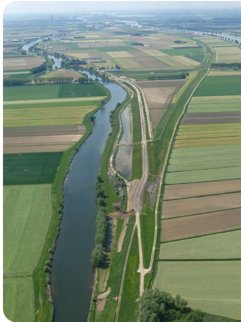
The Overdiepse Polder, one of over 30 Room for the River projects run by Rijkswaterstaat, where the river was widened in order to enlarge the drainage capacity during high water.
